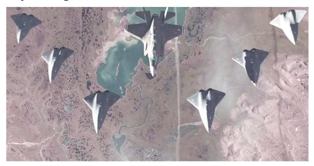
The F-35 is on its way to becoming the new aerial combat platform. The Loyal Wingman, a program whereby a single F-35 is accompanied by several AI powered drones, is gaining steam. The drones which cost a lot less than the F-35 could take a hit for the F-35, jam radars, carry extra launch weapons, and scout ahead.
